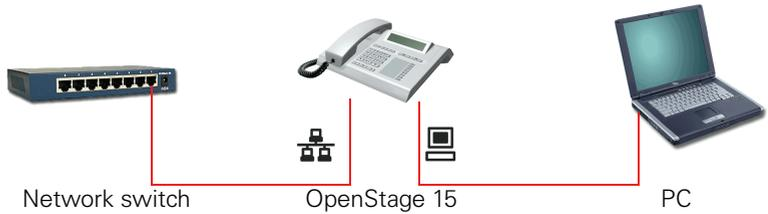
Using this connection option saves one network port for each switch used and requires fewer or shorter network cables when arranged correctly.
